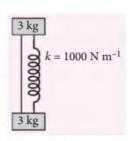
certain moment. At what minimum value of initial compression  $x_0$  (in cm) of the spring will the lower cube bounce up after the thread is burnt through?
